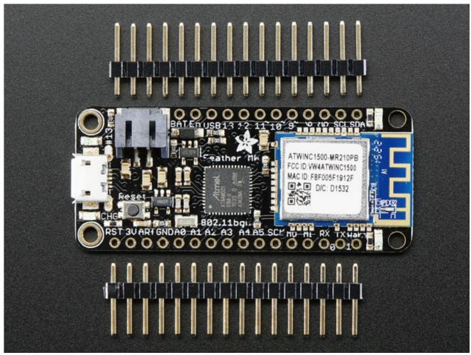
Comes fully assembled and tested, with a USB bootloader that lets you quickly use it with the Arduino IDE. We also toss in some header so you can solder it in and plug into a solderless breadboard. Lipoly battery (http://adafru.it/e0v) and MicroUSB cable (http://adafru.it/aM5) not included (but we do have lots of options in the shop if you'd like!)
