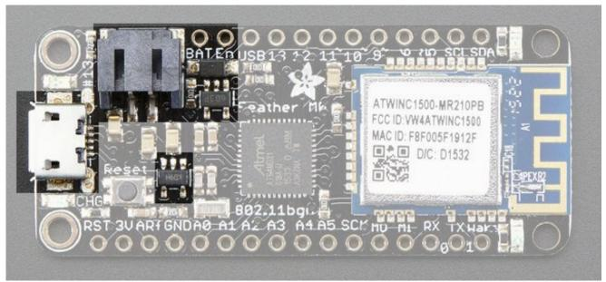
The above shows the Micro USB jack (left), Lipoly JST jack (top left), as well as the 3.3V regulator and changeover diode (just to the right of the JST jack) and the Lipoly charging circuitry (to the right of the Reset button). There's also a **CHG** LED, which will light up while the battery is charging. This LED might also flicker if the battery is not connected.
