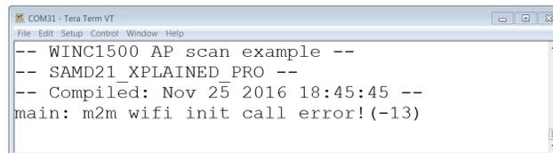
Setting the `CONF_WIFI_DEBUG` to '1' in the `conf_winc.h` configuration file of the host application project provides more information about the version mismatch error.
