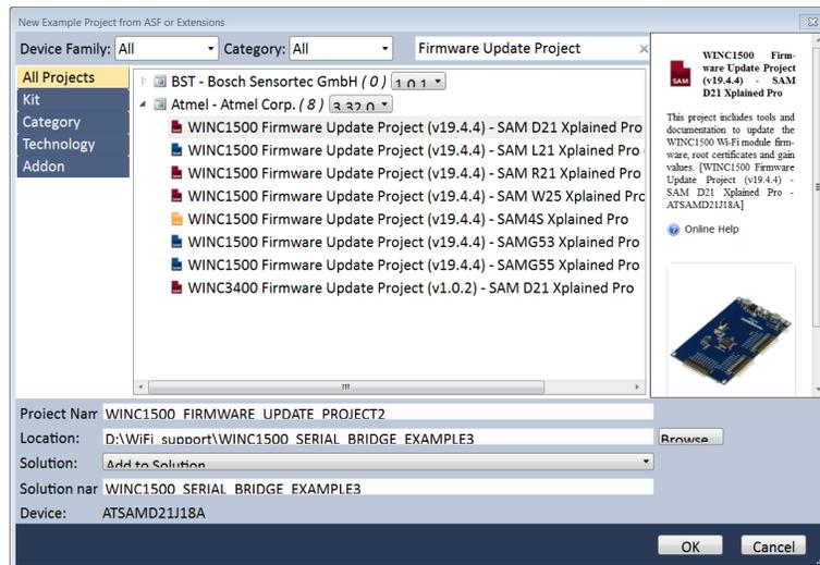
2. Select the appropriate "WINC Firmware Update Project (vxx.x.x)" corresponding to the intended host MCU Xplained Pro board and then press the **OK** button to import firmware update project and related documentation.
