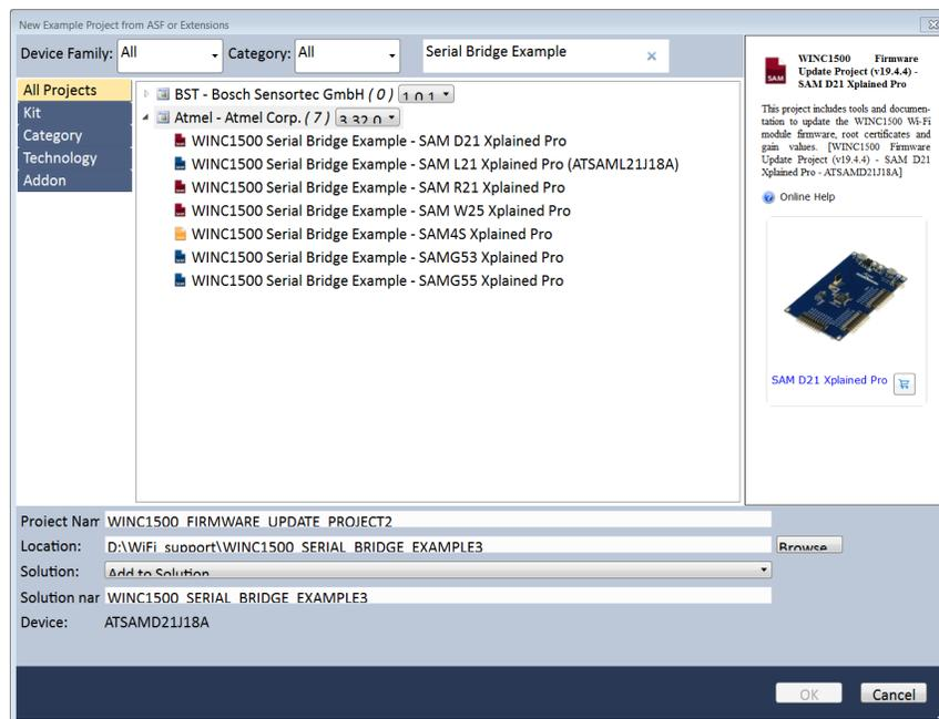
2. Select the appropriate “WINC Serial Bridge Example” project corresponding to the intended host MCU Xplained Pro board and then press the **OK** button to import the project and related documentation.
