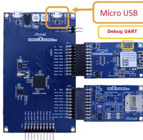
When a Micro-USB plug is not present on the WINC-Xpro board, the RX, TX, and GND UART signals (see [Table 3-1](#)) that are available on the board can be connected to a PC using a third-party serial-to-USB converter.
